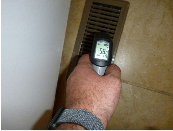
Cooling: View of supply air temperature using a digital thermometer in the cooling mode
